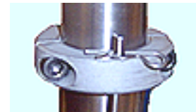
The cotter pin secures the clevis pin.
