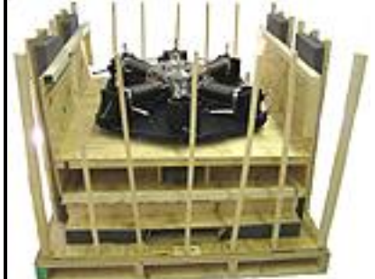
Shipping fixture after removing top and two sides
